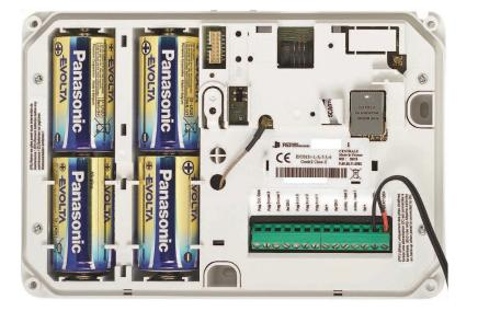
In this functioning mode, the XT-iP panel works as a standard hybrid alarm system with 25 wireless peripherals and 3 programmable inputs. It is a totally standalone alarm system.
