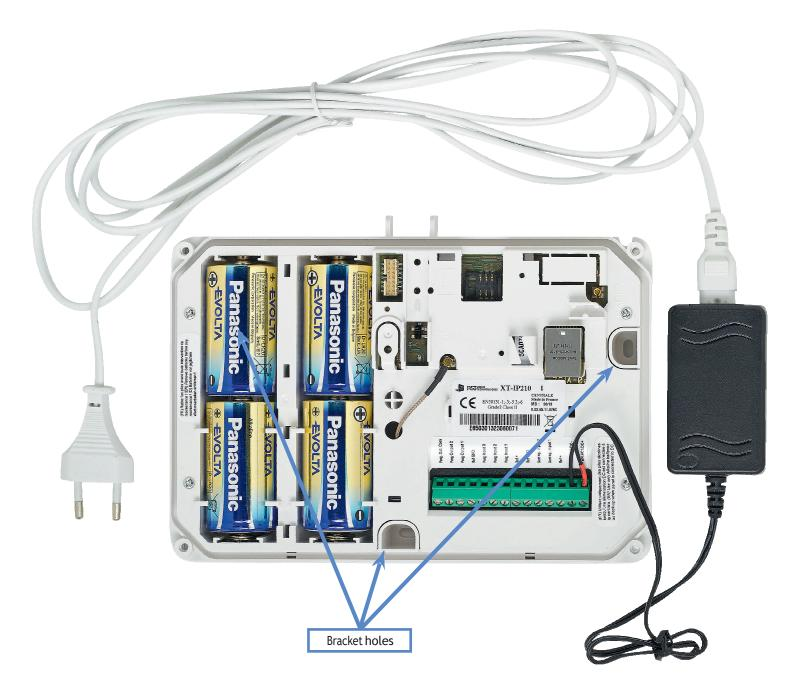
Mount the rear case on the wall using the three mounting holes illustrated above. Mounting the panel is not required for programming.
