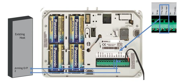
When the XT-IP panel is used in XTENDER mode, the system will only be able to arm and disarm by latching 9-12Vcc to its arming inputs Arming Input 1 and/or Arming Input 2.
